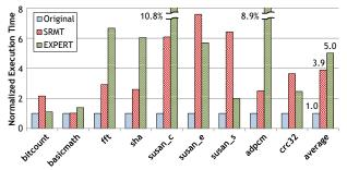
**Fig. 5:** EXPERT-protected programs run 30% slower than SRMT-protected ones.
