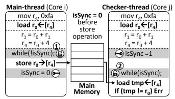
Fig. 2: EXPERT transformation runs two copies of a program thread and synchronize them on store operations. Main thread performs store and the checker thread verifies the correct execution of store by loading the written value from memory and check it against its own locally computed one.
