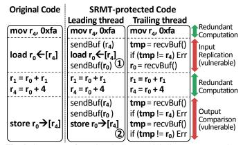
**Fig. 1:** SRMT transformation duplicates original program execution thread. Only leading thread performs memory operations. Trailing thread validates the correctness of memory instruction register operands while the execution of memory operations themselves remains unprotected.
