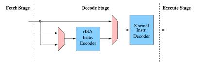
Fig. 4. Two step Decoding of Thumb instructions
