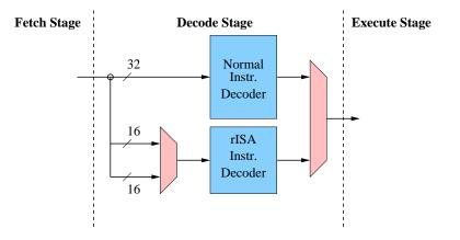
Fig. 3. Single step Decoding of rISA instructions
