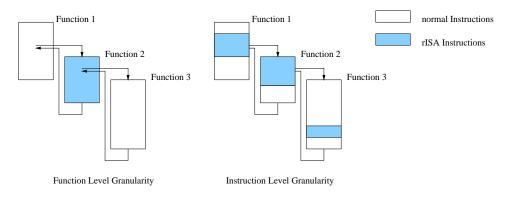
Fig. 6. Routine Level Granularity versus Instruction Level Granularity
