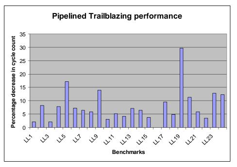
Figure 15: Change in performance after enabling Pipeline Trailblazing
