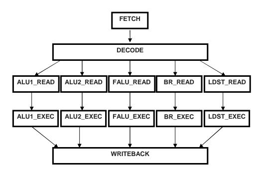
Figure 1: Simplified acesMIPS architecture
