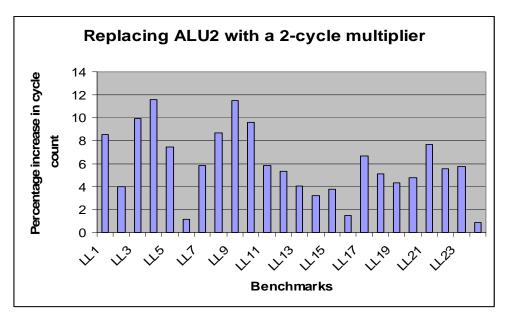
Figure 18: Change in performance after replacing ALU2 with 2-cycle multiplier
