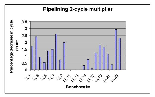
Figure 19: Change in performance after pipelining multi-cycle multiplier
