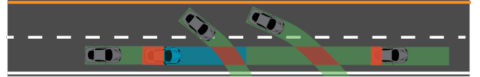
Fig. 11: BlaFT (blue car) is in LF-mode in the hybrid traffic. It is safe from the front car (the rightmost red rectangle) by lemma 1. When it comes to the other vehicles from adjacent lane and the behind (the remaining red ones), BlaFT has the right-of-way. For this reason, if the accident came from the adjacent lane(s) or behind, BlaFT remains blame-free .
