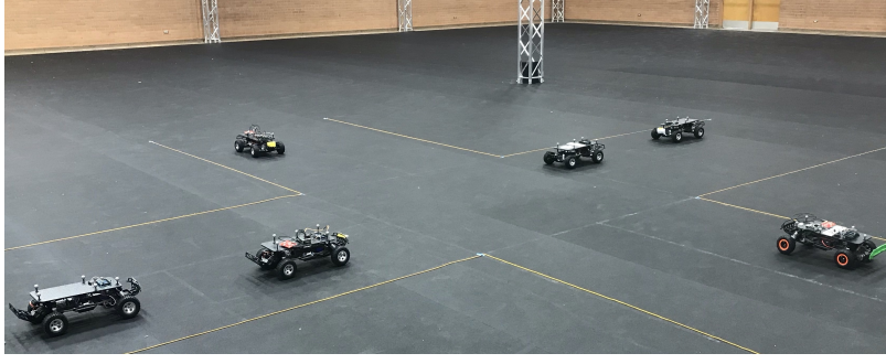
Figure 7.3: Autonomous Intersection Manager Using Traxxas Cars.
