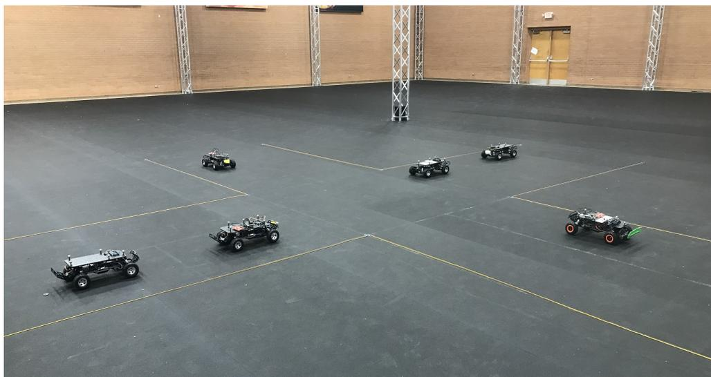
Figure 5.2: Our Testbed Is a Single-lane Intersection with 1/10 Scale Model CAVs. CAVs Position is Tracked by the OptiTrack System.
