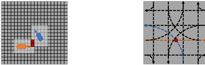
(a) The grid represents the areas that will be occupied by vehicles at time t . A conflict exists if two areas have an overlap (depicted in red). (b) Predefined paths are defined for crossing the intersection. A conflict exist if two paths cross and the cross times of the vehicles overlap.
