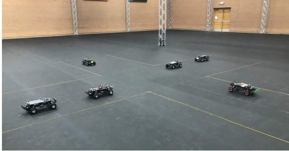
Fig. 2. Our testbed is a single-lane intersection with 1/10 scale model CAVs. CAVs position is tracked by the OptiTrack system.
