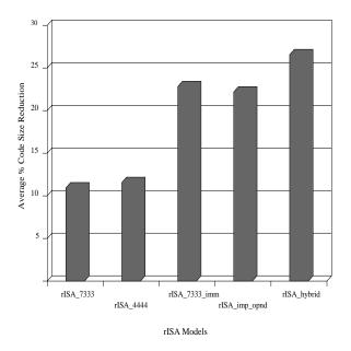
Figure 3: Code size reduction for various rISA architectures
