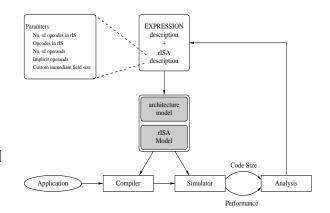
Figure 1: Design Space Exploration flow
